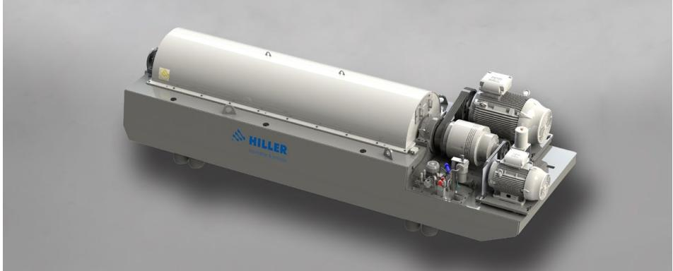
As the clarified liquid flows along the bowl towards the liquids discharge zone, the centrifugal force causes the light and heavy liquid phases (typically oil and water) to separate; the oil moving upwards to the rotating axis and the water gathering in the middle between the oil and the sediment layers.
